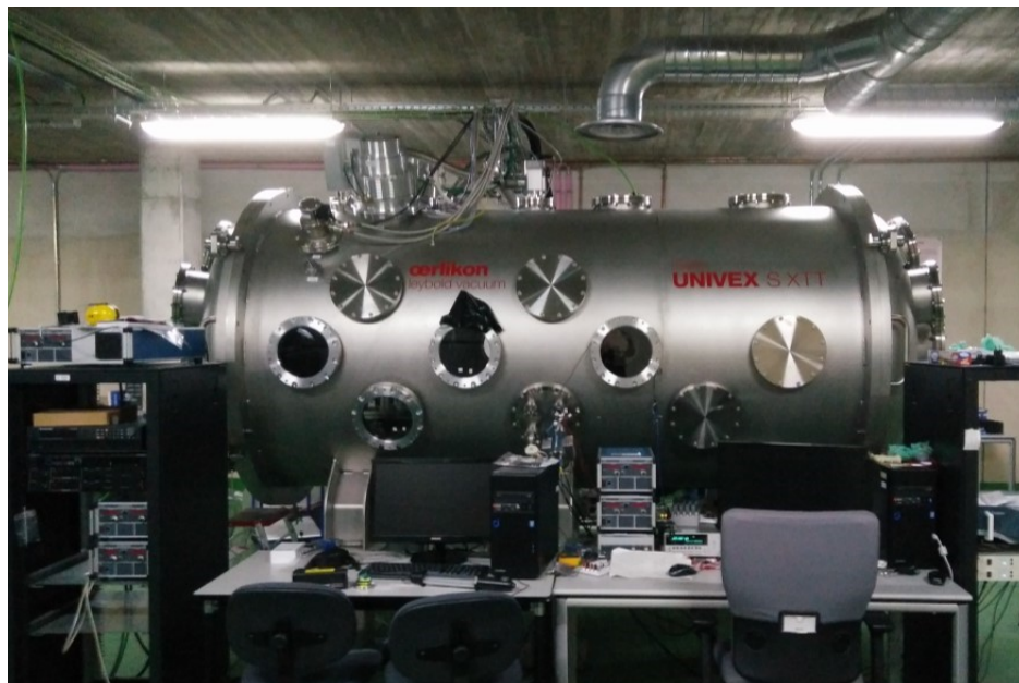
Figure 2. Vacuum chamber in the EP2 Space Propulsion Laboratory, UC3M (Madrid).
