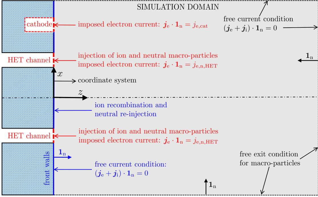
Figure 1. Boundary conditions for both the PIC macro-particles and the fluid electrons, in the considered simulation scenario. The neutralizer is depicted in a lateral position for the sake of clarity, although the nominal case simulation considers a neutralizer at the thruster axis, as reported in Tab. 1.
