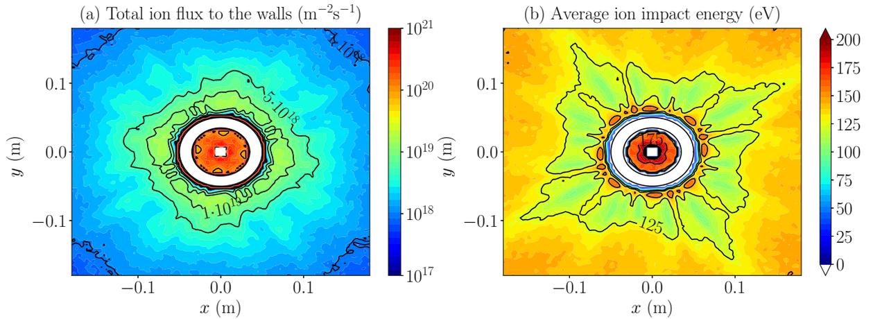
Figure 5. (a) Ion flux and (b) mean impact energy on the front walls of the HET.
