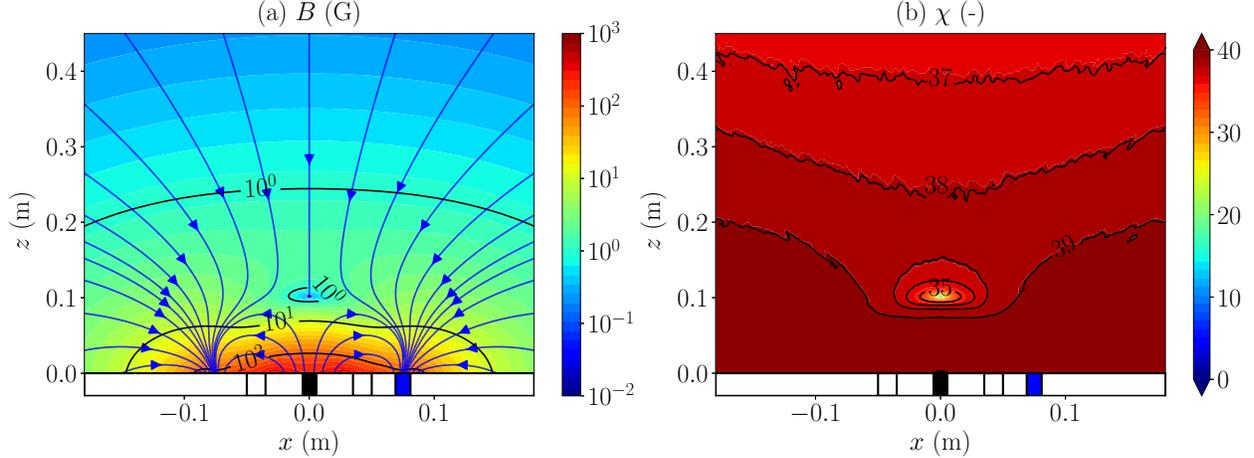
**Figure 3.** Nominal simulation results at  $y = 0$  showing: (a) magnetic field magnitude and streamlines, and (b) Hall parameter. The projection of the thruster and annular channel walls with the  $x - z$  plane are shown by the black solid lines at  $z < 0$ , while the neutralizer is indicated by either a black (symmetric cases) or blue (asymmetric case) rectangle.
