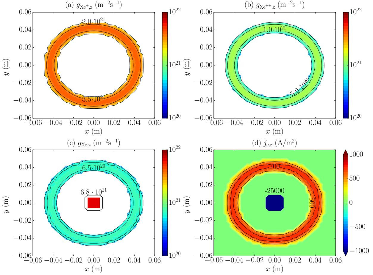
**Figure 2.** Imposed injection fluxes at  $z = 0$  for (a) singly-charged ions, (b) doubly-charged ions, (c) neutrals, and (d) normal electron current density at  $z = 0$ . For these plots, a centerline neutralizer is considered. The side of the neutralizer emission area is 1.2 cm, equivalent to 4 PIC cells.
