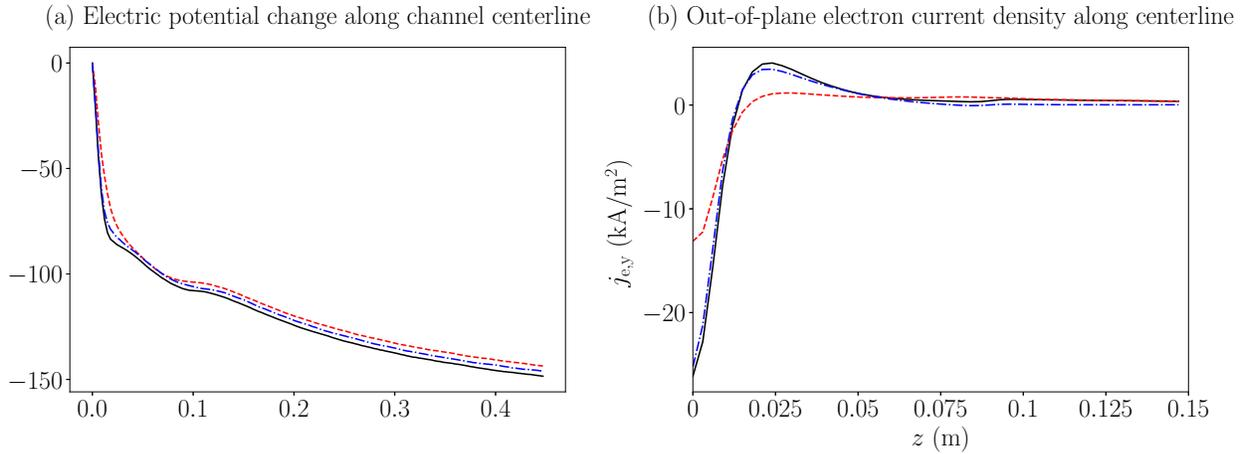
**Figure 7.** Comparison of nominal simulation ( $\alpha = 0.025$ , black solid lines), higher anomalous transport simulation ( $\alpha = 0.05$ , red dashed lines) and lateral neutralizer simulation ( $\alpha = 0.025$ , blue dash-dot lines) showing the 1D evolutions of: (a) electric potential change, and (b) aximuthal electron current density along the HET channel centerline.
