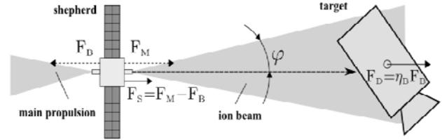
Figure 1. Schematic of the IBS concept.
