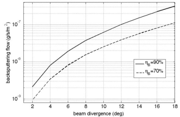
**Figure 3.** Backsputtering flow reaching the IBS spacecraft from an aluminium spherical target with constant momentum transfer efficiency and varying beam divergence.
