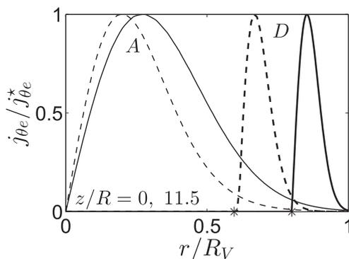
FIG. 7. Azimuthal electron currents (normalized with maximum value of each curve) for simulations A (thin) and D (thick). The dimensionless peak values are 5.46 at  $z=0$  (solid) and 0.34 at  $z/R=11.5$  (dashed) in simulation A, and 26.6 at  $z=0$  and 0.71 at  $z/R=11.5$  in simulation D. Asterisks correspond to the same points of Fig. 1(b).
