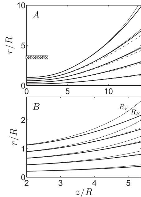
FIG. 2. Streamtubes of magnetic field (solid, thick), electrons (solid, thin), and ions (dashed) for simulations A and B. Each group of 3 lines starts from the same location at  $z = 0$ , thus showing the downstream electron and ion separation from the magnetic field.  $R_V$  and  $R_B$  represent the beam and nozzle edges, respectively. The electron separation of simulation A is the same as that of C. Notice the different axes scales.
