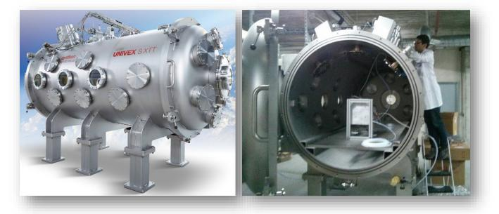
The 200  $m^2$  laboratory hosts, among other facilities, a large stainless steel vacuum chamber built and certified by Leybold Oerlikon and optimized for the testing of low-mid power Hall effect, gridded ion, and RF thrusters (helicon, ECR) up to about 2 kW and 100 sccm:
